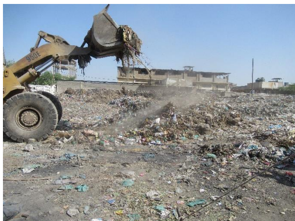
Exhibit 2.3: Mixing of Waste with the help of Loader
