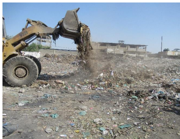
Exhibit 2.4: Mixing of Waste with the help of Loader
