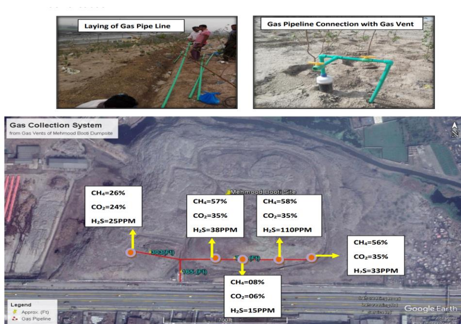
Figure 4.5: Pictorial presentation of Landfill Gas Capturing Process
